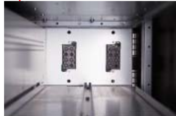
FEMALE CONNECTORS FOR BATTERY MODULES
